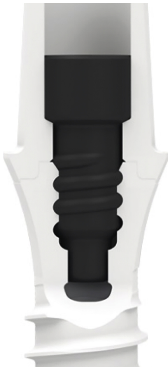
Fig. 1. Schematic cross-section of the all-ceramic 2-piece zirconia implant | abutment system with carbon-fiber reinforced polymer screw (Zeramex P6 Implant, Zerafix Abutment + Screw, Dentalpoint AG, Zurich, Switzerland).
