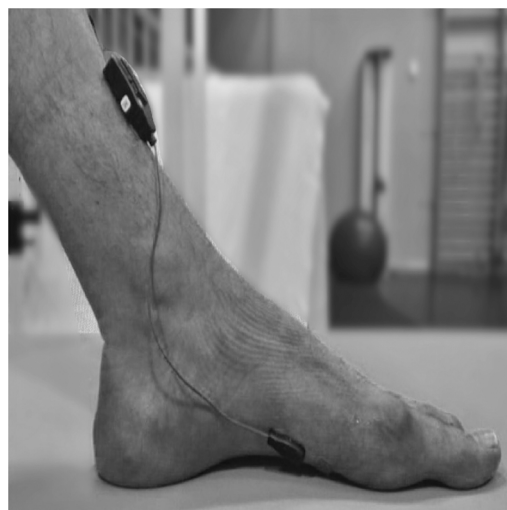
Fig. 1. Trigno Mini wireless sensor placed on the foot for abductor hallucis muscle.
