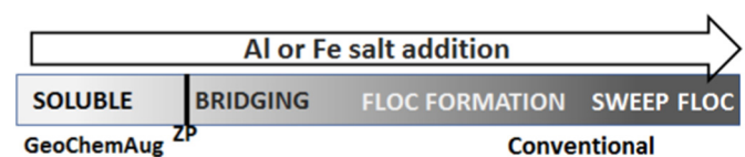
Fig. 1. Schematic dosing definition of geochemical augmentation. Dosing is always less than particle's neutral zeta potential (ZP), which is the charge neutralization threshold for floc formation.
