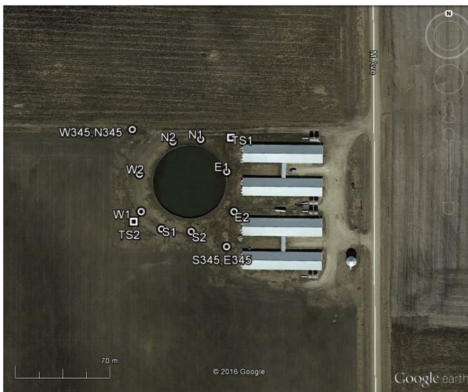
Fig. 1. Configuration of study site. Locations of the five retroreflectors on each cardinal direction from the tank are indicated with a prefix of direction from the tank. Retroreflectors 3, 4, and 5 were mounted on towers while 1 and 2 were on tripods. Scanning TDLAS units are indicated by 'TS'. Image from GoogleEarth®.
