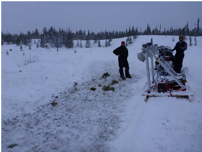
Fig. 1. Example of bare soil site and the surface-based radiometers on a mobile sled.
