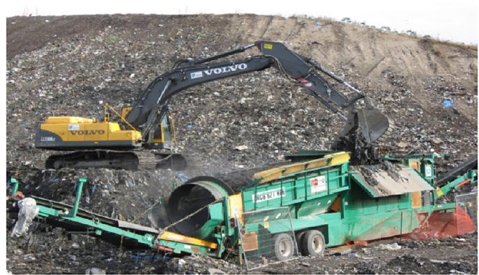
Fig. 1. Photographs showing the landfill soil reclamation process: material post screening (left) and screening plant (right).
