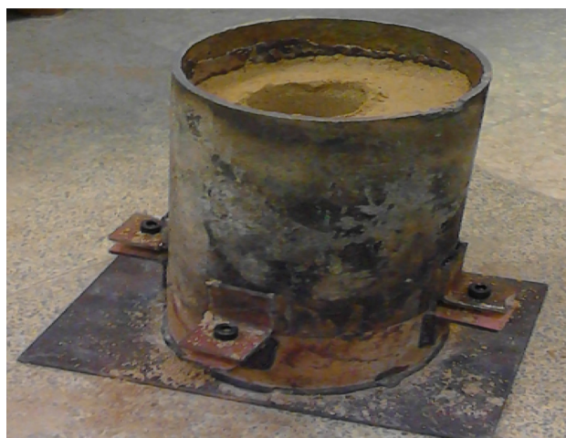
Fig. 2. The magnesia-lined steel reactor for the SHS process.
