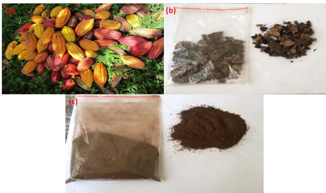
Fig. 1. (a) samples of cocoa pods, (b) dried cocoa pod husks, (c) milled cocoa pod husks.
