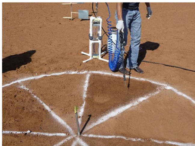
Fig. 2. Application of the erbium nitrate solution to an octant of the 5 m 2 source area.
