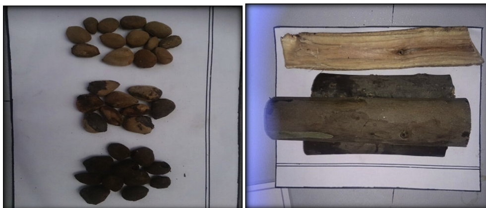
Fig. 1 – Marula seeds (left) and Blue gum tree wood (right) used for torrefaction studies.
