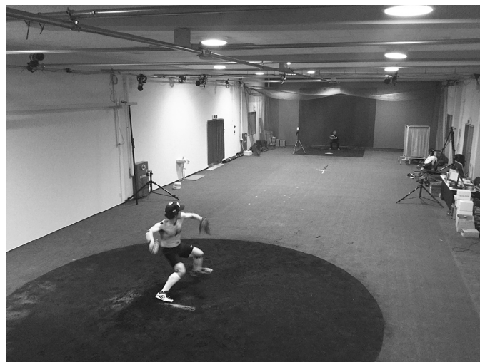
Figure 2 Three-dimensional positions of the markers during throwing motion were recorded by the charge-coupled device cameras.
