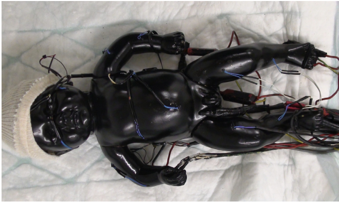
Fig. 1. Thermal mannequin representing an newborn with a body weight of 1800 g.
