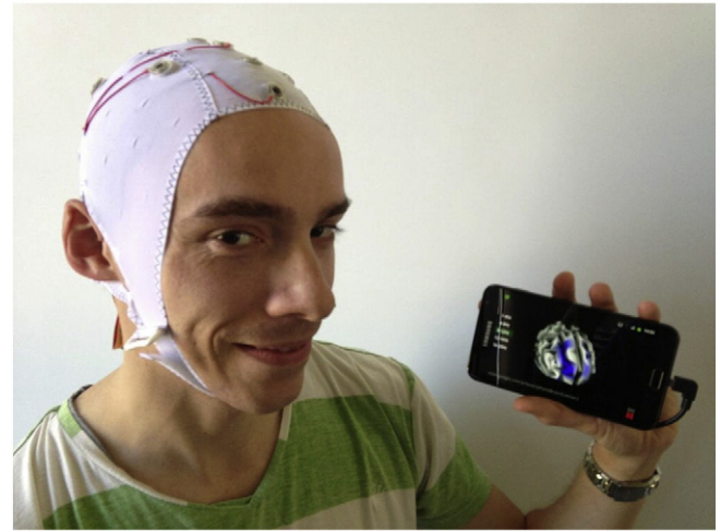
Fig. 1. SBS2 mobile EEG recording with real-time 3D source reconstruction, on an Android smartphone connected wirelessly to an Easycap 16 electrode setup based on Emotiv hardware.
