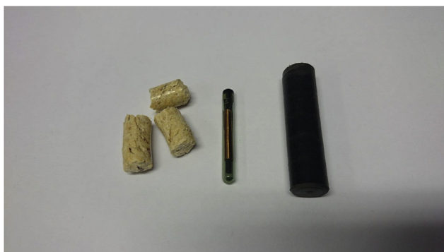
Fig. 1. RFID tag and hard shell.
