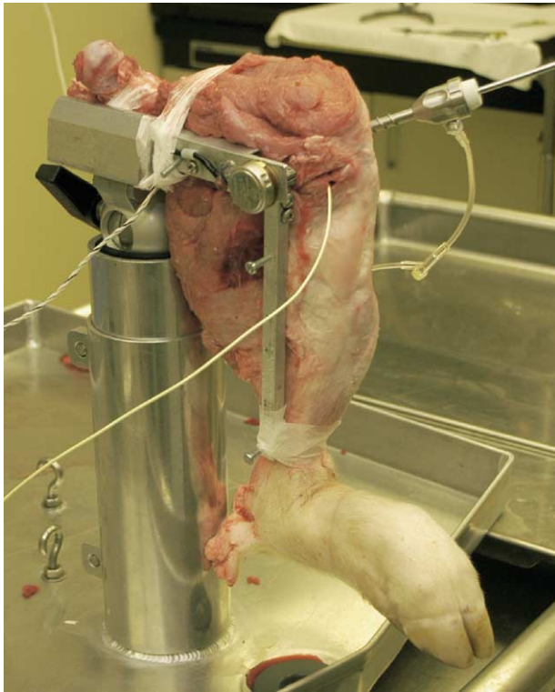
FIGURE 1. The pig legs were clamped in a stand with an electronic goniometer centered at the lateral joint line and secured to the femur and fibula. The goniometer was wired into the computer workstation, allowing kinematic analysis of the porcine knees. The arthroscopic visualization was done through the anterior medial portal and a pressure transducer was placed into the meniscal tear through the anterior lateral portal.
