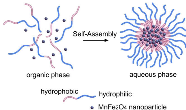
Scheme 1. Schematic illustration of mPEG- b -PCL/Mn-SPIO micelle formation and Mn-SPIO nanocrystal clustering inside the micelle core.
