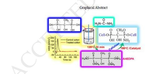
An efficient flame retardant AHEDPA for cotton was obtained through one-step clean synthesis using obtainable.
