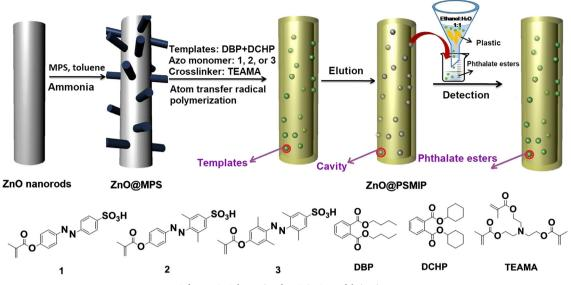
Scheme 1. Schematic of ZnO@PSMIP fabrication.
