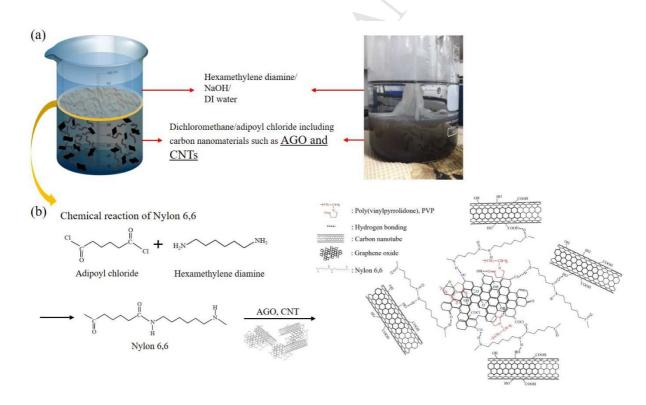
(a) Schematic of *in-situ* interfacial polymerization process of nylon 6,6 including AGO, CNT with PVP showing (b) chemical reaction of nylon 6,6 synthesis and its occurrence at the interface between two immiscible phases is demonstrated in inset photograph of (a).
