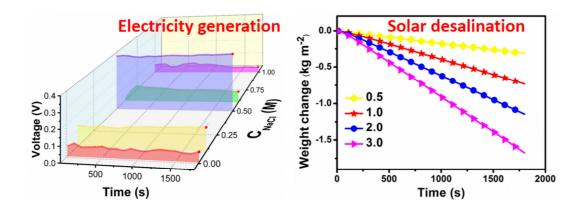
A graphene/carbon cloth device is fabricated to generate electricity approximately up to 0.37 V in 0.5 M NaCl solution through solar-driven water evaporation.
