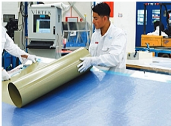
Fig. 2. Layup process for panels made from GLARE. (For interpretation of the references to colour in this figure legend, the reader is referred to the web version of this article.)
