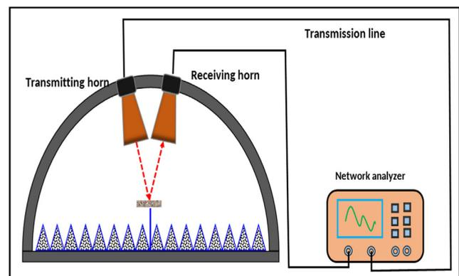
**Fig. 1.** Sketch map of the arch reflecting method system.
