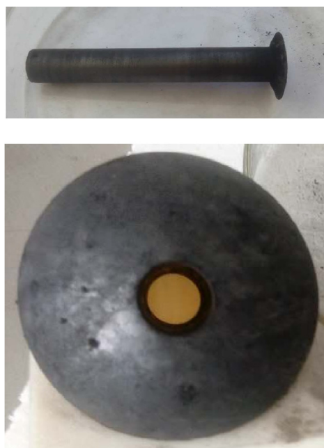
Fig. 1. Cylindrical graphite stick sample drilled from the irradiated graphite sphere of HTR-10.
