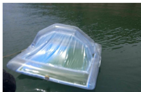
Fig. 2. Photograph of the used floating PBR (1 m 2 ).
