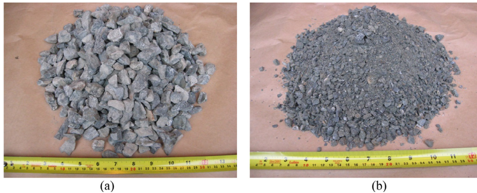
Fig. 2. (a) Pre-crushed rock feed and (b) crushed product.
