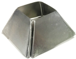
Fig. 1. Sample of a single unit of truncated square pyramid folded from aluminium sheet (hand folded).
