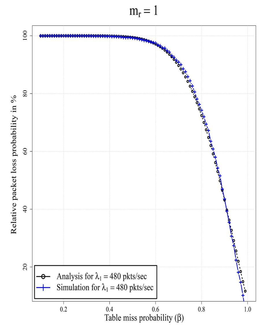
Relative packet loss probability between Software and Hardware Switch
