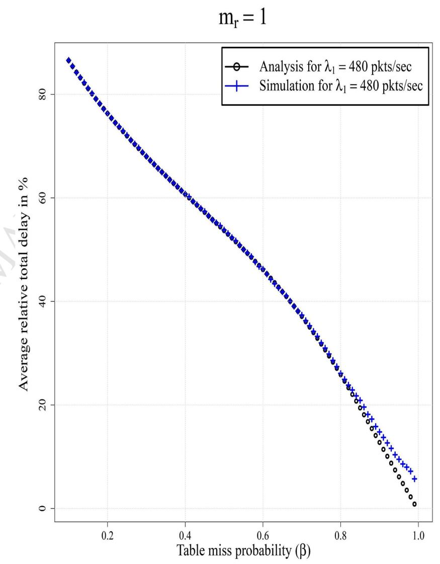
Relative average packet delay between Software and Hardware Switch
