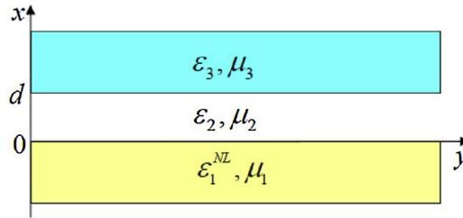
Fig. 1. Schematic structure of the metal waveguide with a nonlinear substrate and a linear cladding, the core thickness is  $d$ . (For interpretation of the references to color in text/this figure legend, the reader is referred to the web version of the article.)
