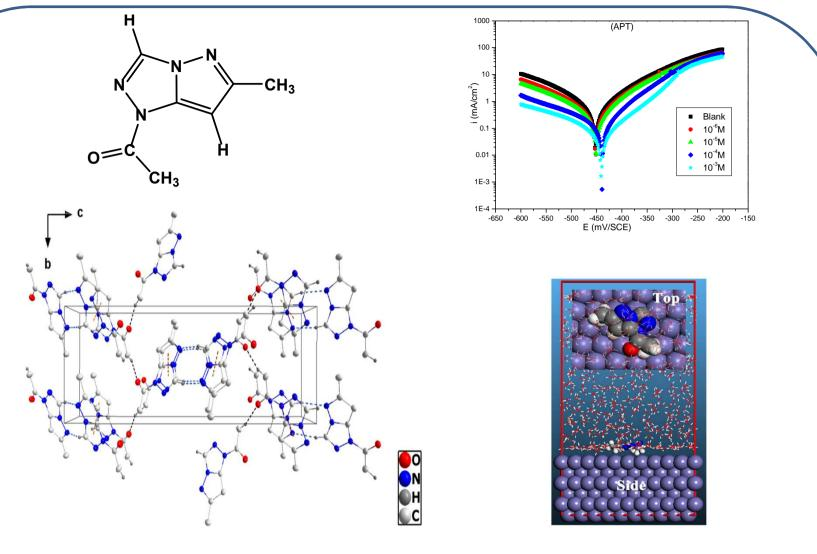
2D structure (up right), molecular packing (bottom right), Polarization curves for carbon steel in the absence (blank) and presence of APT at different concentrations (up left) and MD simulation of APT on Fe surface (bottom left).
