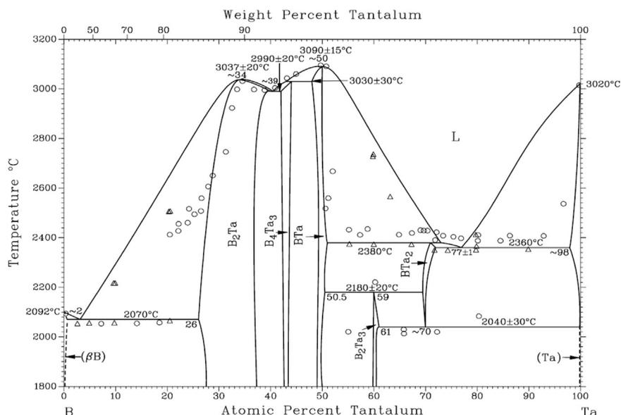
Fig. 1. Currently accepted phase diagram of the Ta-B system [3] along with experimental data from: ○ Rudy [4] and △ Portnoi et al. [5].
