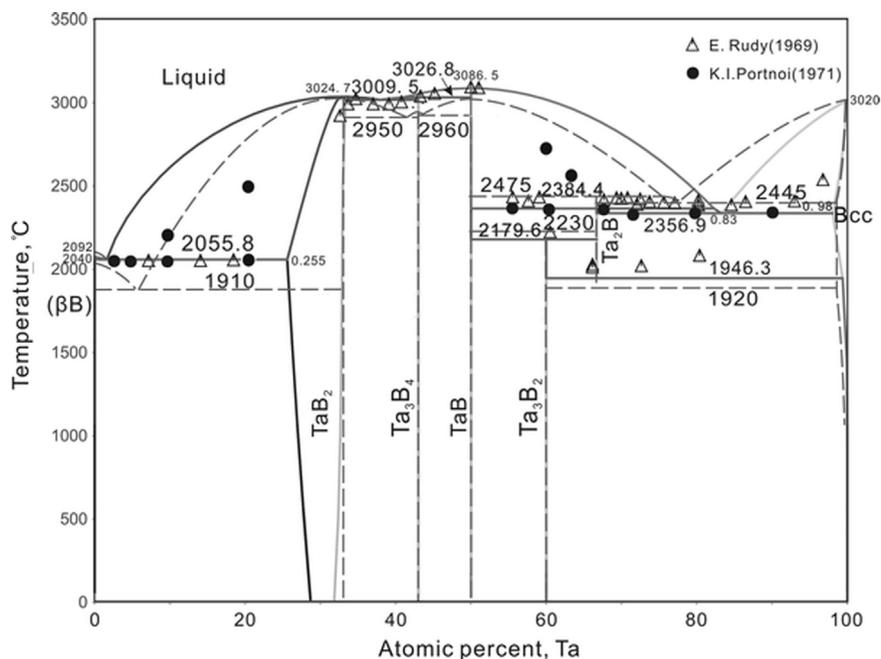
Fig. 2. Ta-B phase diagram published by Yang et al. [19] calculated with their parameters (solid lines) and Kaufman's [20] (dotted lines) along with selected experimental data from Rudy [4] and Portnoi et al. [5].
