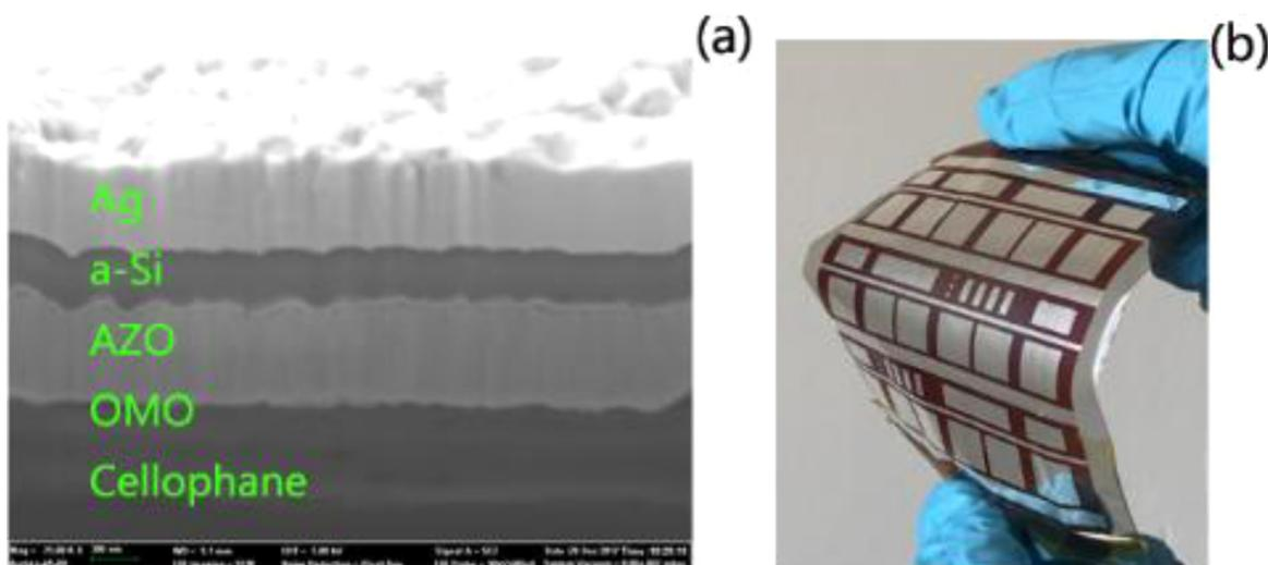
Fig. 1. (a) Cross sectional FIB-SEM image and (b) picture of a-Si:H solar cells on cellophane substrate.
