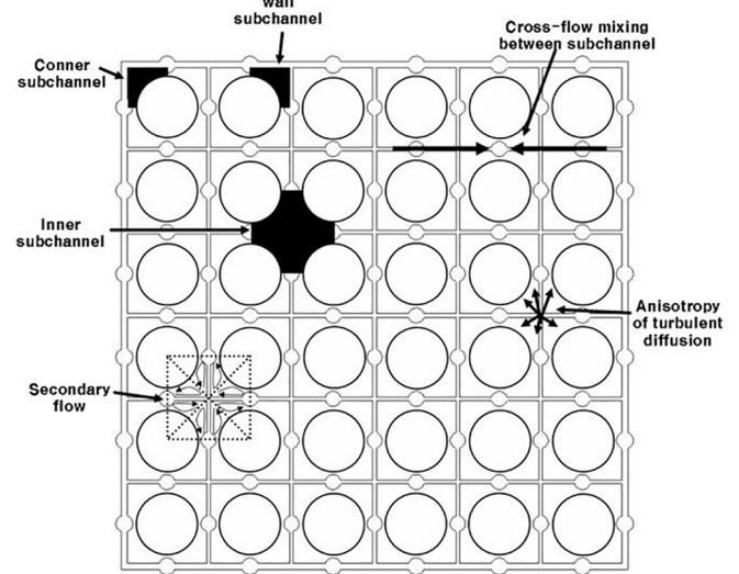
Fig. 2. Configuration and secondary flow phenomena in sub-channel.
