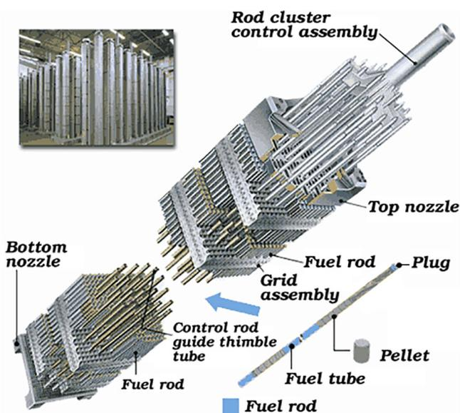
Fig. 1. Typical fuel rod assembly of pressurized light water nuclear reactor.
