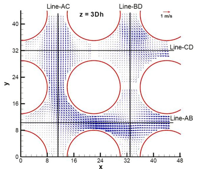
Fig. 3. Lateral vector profile, measured using LDV measurement, in the sub-channels with LSVF mixing vanes (Seo, 2009).
