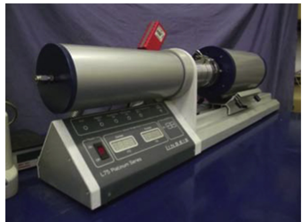
Fig. 1. Push rod facility for thermal expansion coefficient determination.
