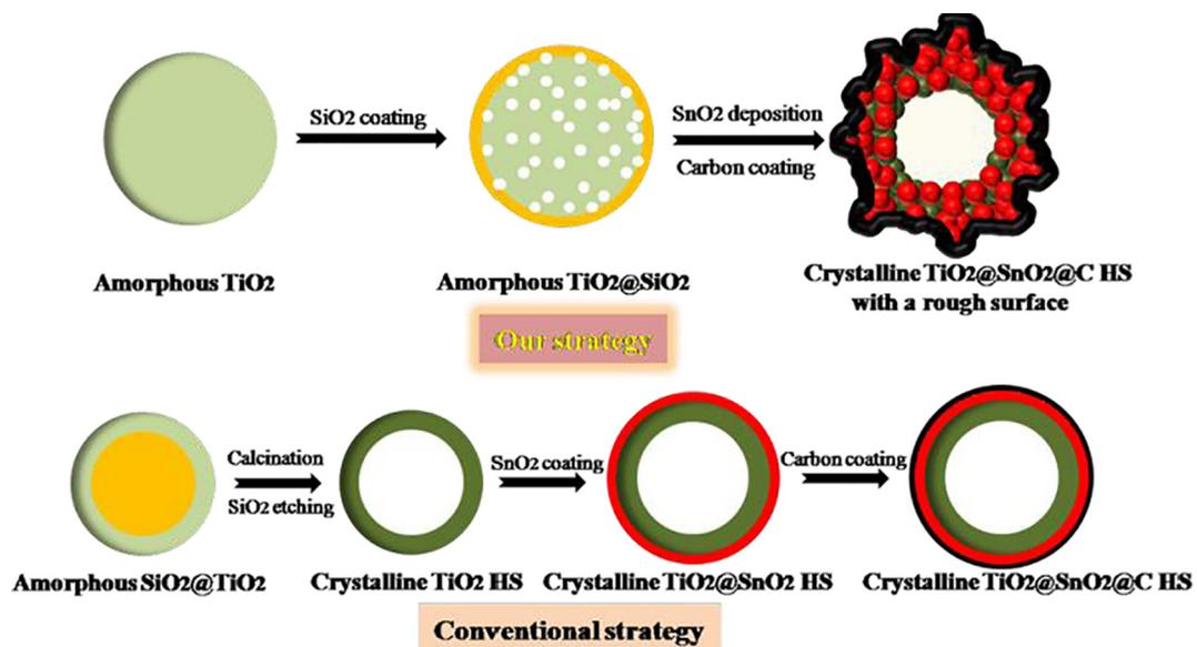
Fig. 1. The preparation schematic of  $\text{TiO}_2@SnO_2@C$  HS.
