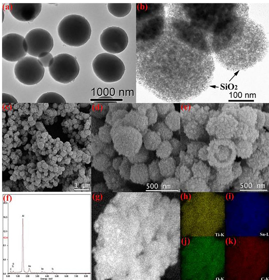
Fig. 2. TEM images of (a)  $\text{TiO}_2$  and (b)  $\text{TiO}_2/SiO_2$ ; (c–e) SEM images, (f) EDX spectrum and (h–k) EDX elemental mappings of  $\text{TiO}_2@SnO_2@C$  HS.
