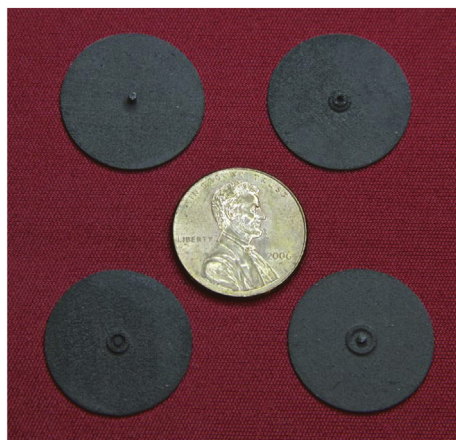
Fig. 1. A photograph of the binderjetted epoxy-infiltrated bonded tungsten filter prototypes: 5 mm cone filter (upper left), 6 mm cone filter (upper right), 8 mm cone filter (lower left), and 10 mm cone filter (lower right).
