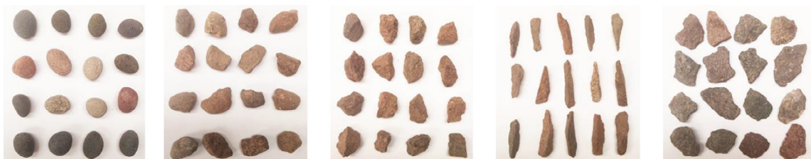
Type I rounded (T1) Type II fractured (T2) Type III angular (T3) Type IV elongated (T4) Type V flat (T5)
