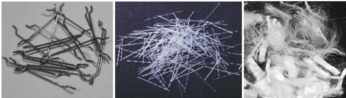
Fig. 1. Photos of fibers used in this study: steel fibers (left), polypropylene fibers (middle), and micro polypropylene fibers (right).
