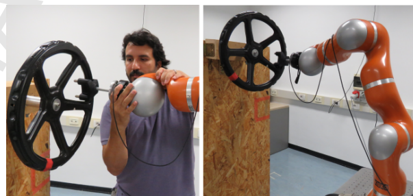
Figure 1: Left : a human operator teaches a robot how to perform a valve-turning task. Right : a snapshot showing the valve-turning task reproduced by a KUKA LWR robot.
