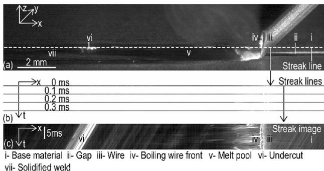
**Fig. 2.** (a) Frame from high speed video, inclined 30°, (b) stacked streak lines (streak line vs. time), and (c) resulting streak image.
