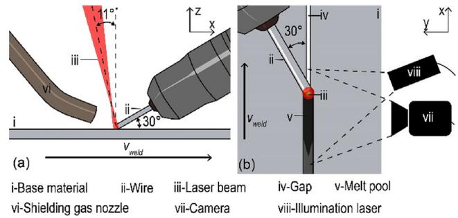
**Fig. 3.** Experimental setup (a) side view, and (b) top view.
