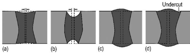
**Fig. 1.** Cross section of welds: (a), (b) without filler wire, where (b) has a larger gap prior to welding; (c), (d) welds with filler wire, where (d) weld has an undercut imperfection.
