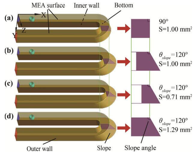
Fig. 1. Computational domain: (a) conventional channel, (b) modified channel with normal sectional area, (c) modified channel with small sectional area and (d) modified channel with large sectional area.
