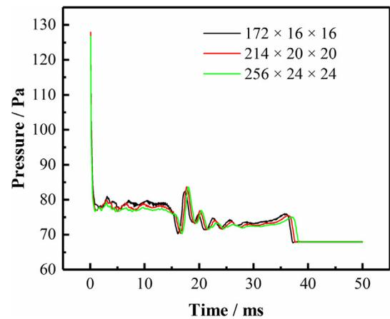
Fig. 2. Results of grid independency test for pressures in the conventional serpentine flow channel with three sets of grid numbers.
