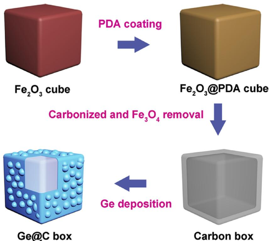
Scheme 1. Illustration of the Ge@C nanobox anodes fabrication process.
