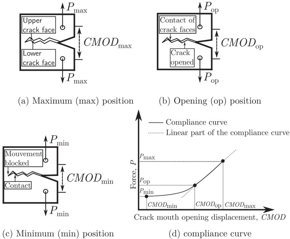
**Fig. 1.** Schematic representation of the roughness-induced crack closure phenomenon and its characterization. (a) At the maximum load, the crack is fully opened. (b) During unloading, a preliminary contact of the crack faces occurs. (c) When the nominal force decreases, the crack tip opening displacement remains constant. (d) Compliance curve ( $P$  versus  $CMOD$ ) used to compute the opening force.
