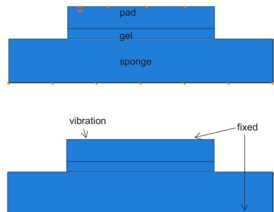
Fig. 2. Geometrical configuration of sponge phantom model.
