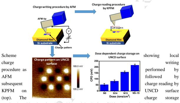
can be altered by changing the tip bias and the doping of N ion implantation (bottom).
