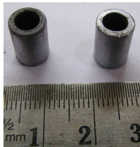
Fig. 4. Tantalum crucibles with TaC coating formed inside, by pack cementation.
