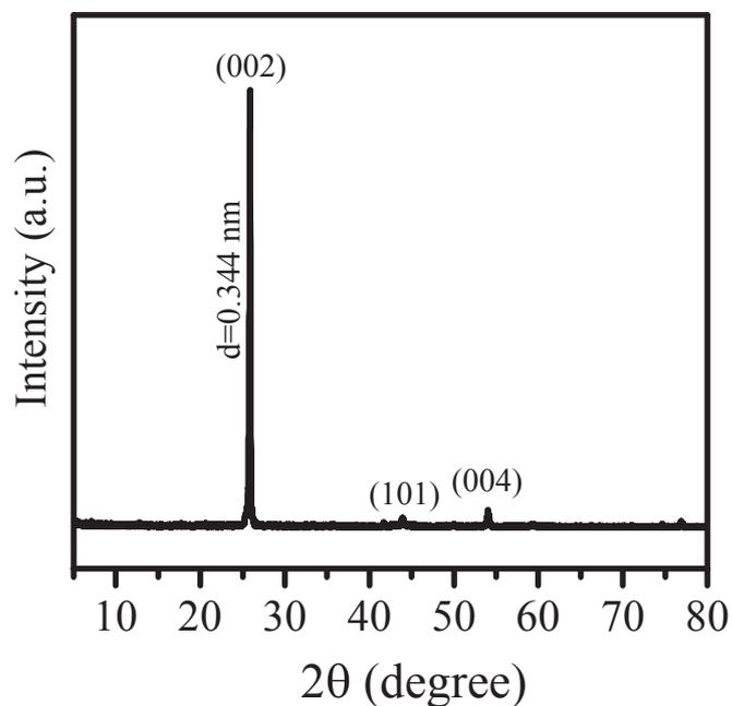
Fig. 1. XRD pattern of the as-processed WG powder.
