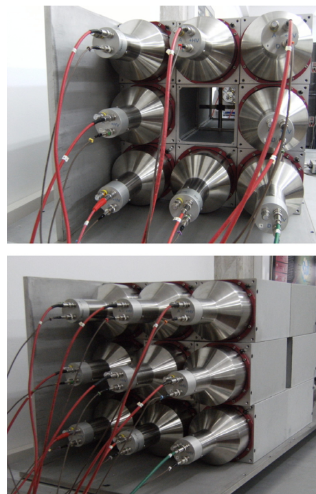
Fig. 1. DTAS detector in the sixteen-module configuration (top) and in the eighteen-module configuration (bottom) without radiation shielding
