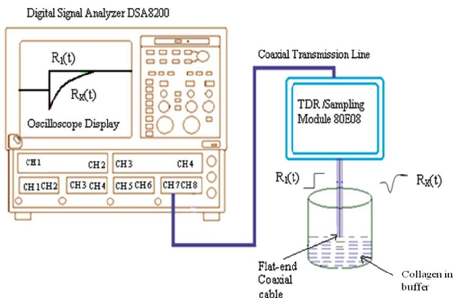
Fig. 1. Experimental setup of time domain reflectometry.
