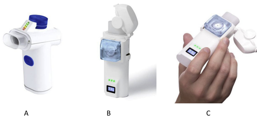
Fig. 1. PneumaHaler digital breath-activated inhaler (A – version used in the described studies, B & C – current version).
