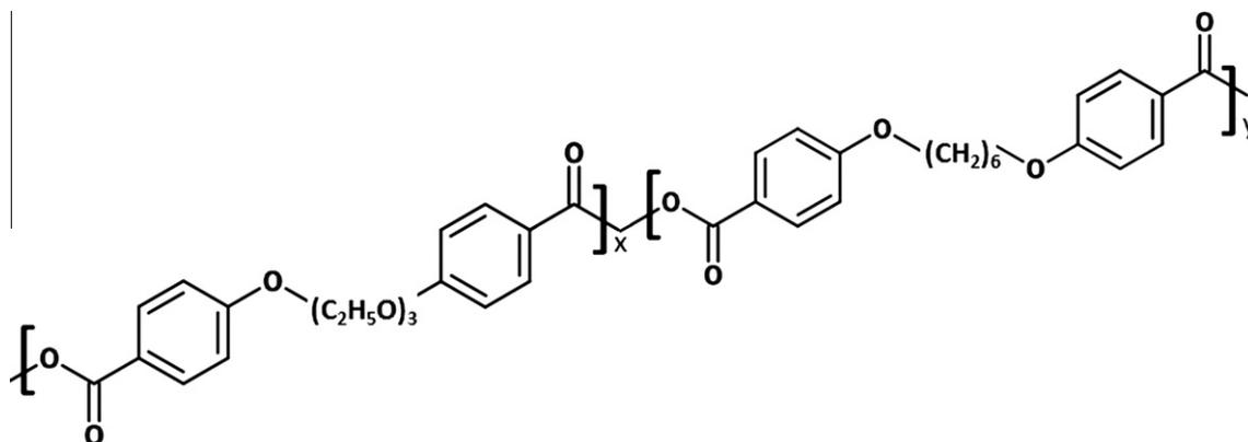
Fig. 1. Chemical structure of CPTEG:CPH polymer.
